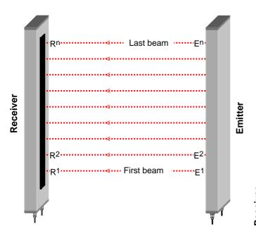
As only the associated receiver of each infrared LED is activated, wide angle radiation is possible. The conical light beams ensure fault-free operation of the **JnfraScan®** photoelectric barriers, even if they are exposed to severe vibration, and greatly simplifies adjustment when mounted.
